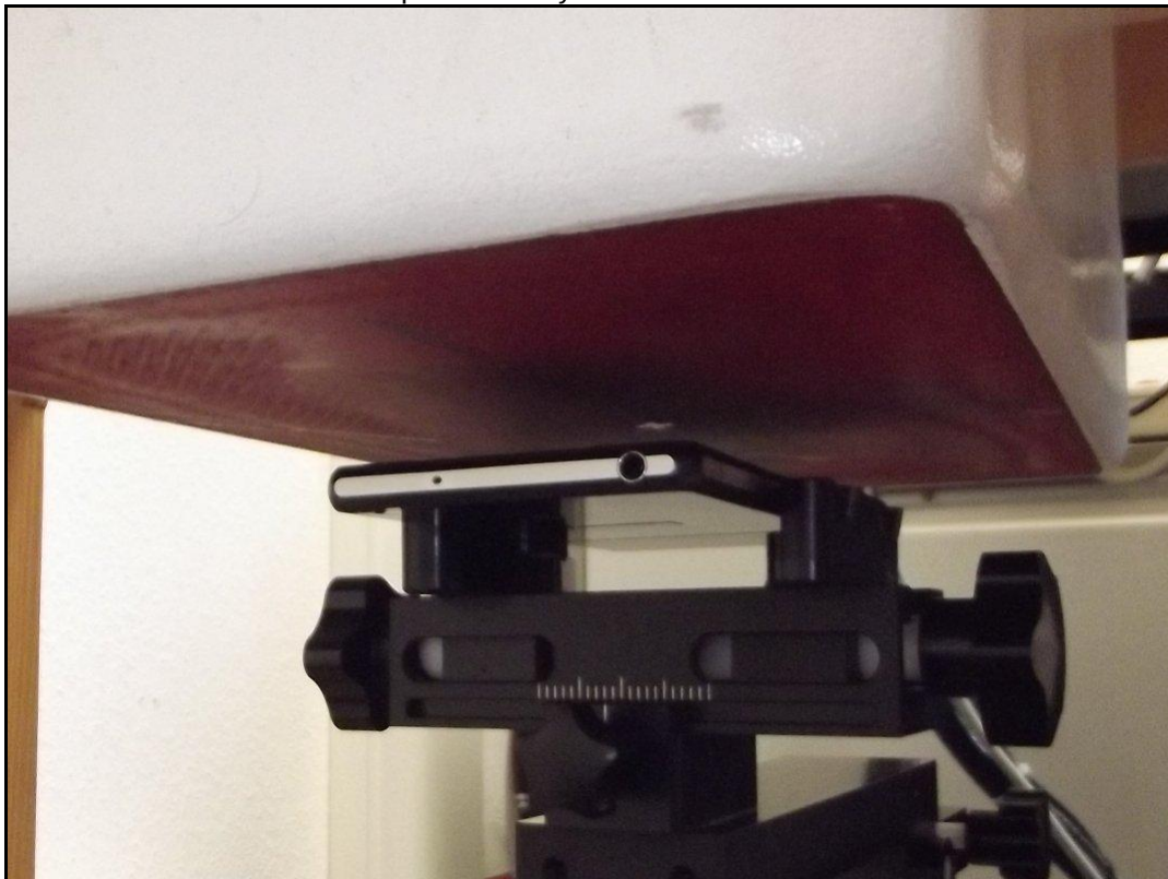
Photo 21: Test position body worn front side 15mm distance
