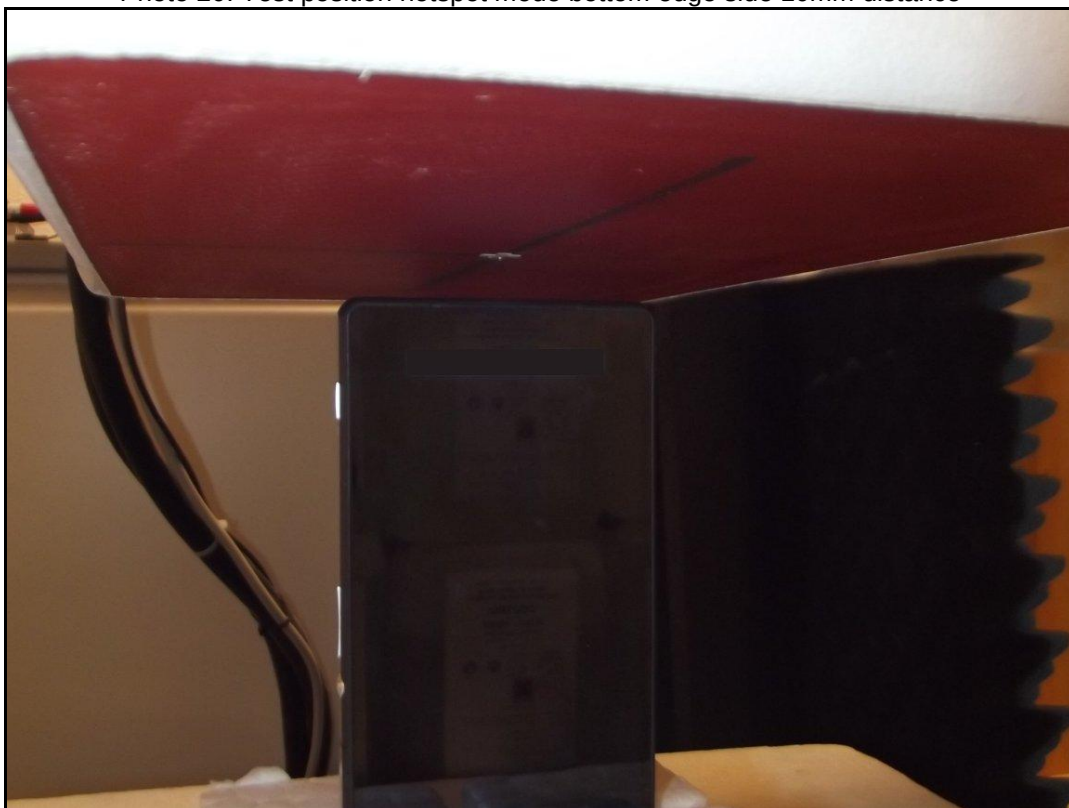
Photo 20: Test position hotspot mode bottom edge side 10mm distance
