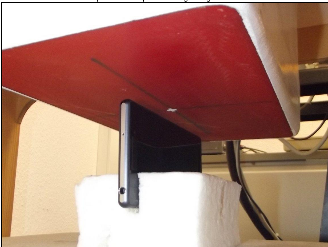
Photo 18: Test position hotspot mode right edge side 10mm distance
