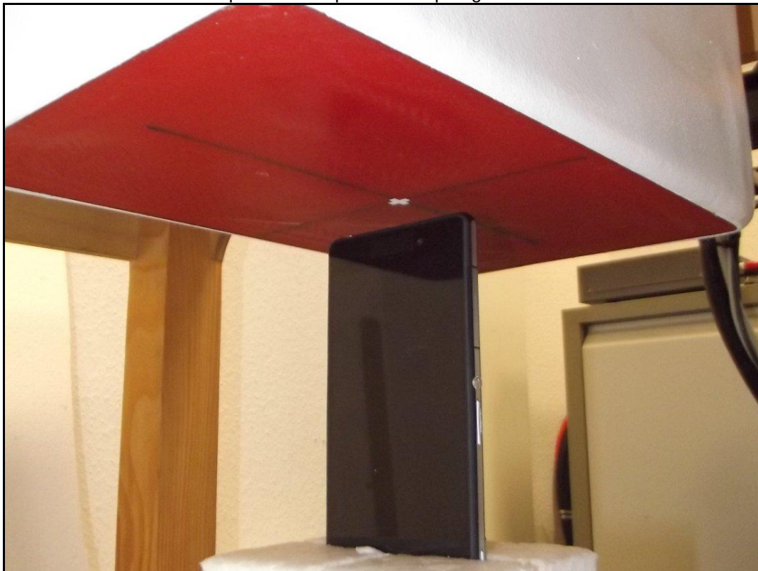
Photo 20: Test position hotspot mode bottom edge side 10mm distance
