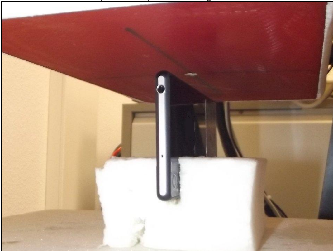
Photo 18: Test position hotspot mode right edge side 10mm distance
