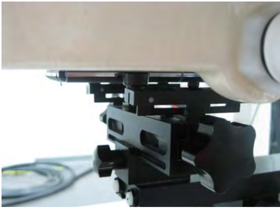
Fig.17 EUT front to flat phantom
