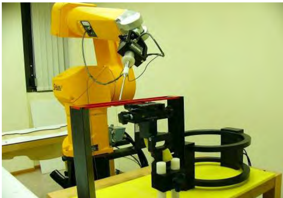
Fig. 1 Photograph of the DASY 5 measurement system
