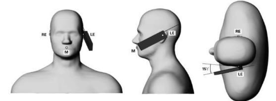
Phone position 2, "tilted position." The reference points for the right ear (RE), left ear (LE) and mouth (M), which define the reference plane for phone positioning.
