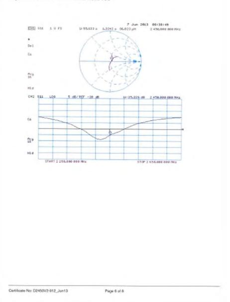
Impedance Measurement Plot for Head TSL
