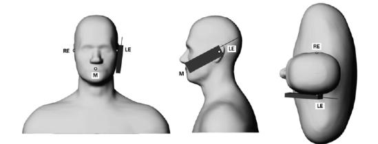
Phone position 1, "cheek" or "touch" position. The reference points for the right ear (RE), left ear (LE) and mouth (M), which define the reference plane for phone positioning.
