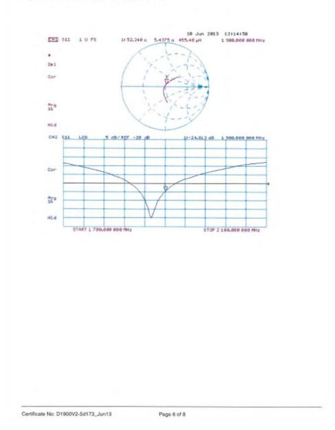
Impedance Measurement Plot for Head TSL
