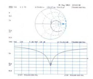
Impedance Measurement Plot for Head TSL
