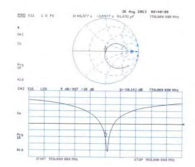
Impedance Measurement Plot for Body TSL
