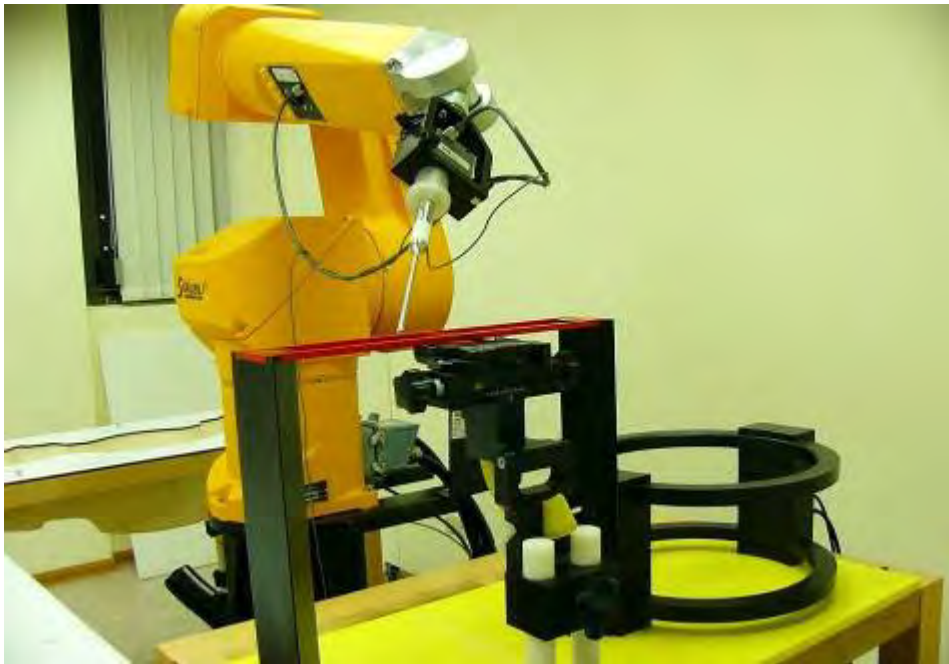
Fig. 1 Photograph of the DASY 5 measurement system
