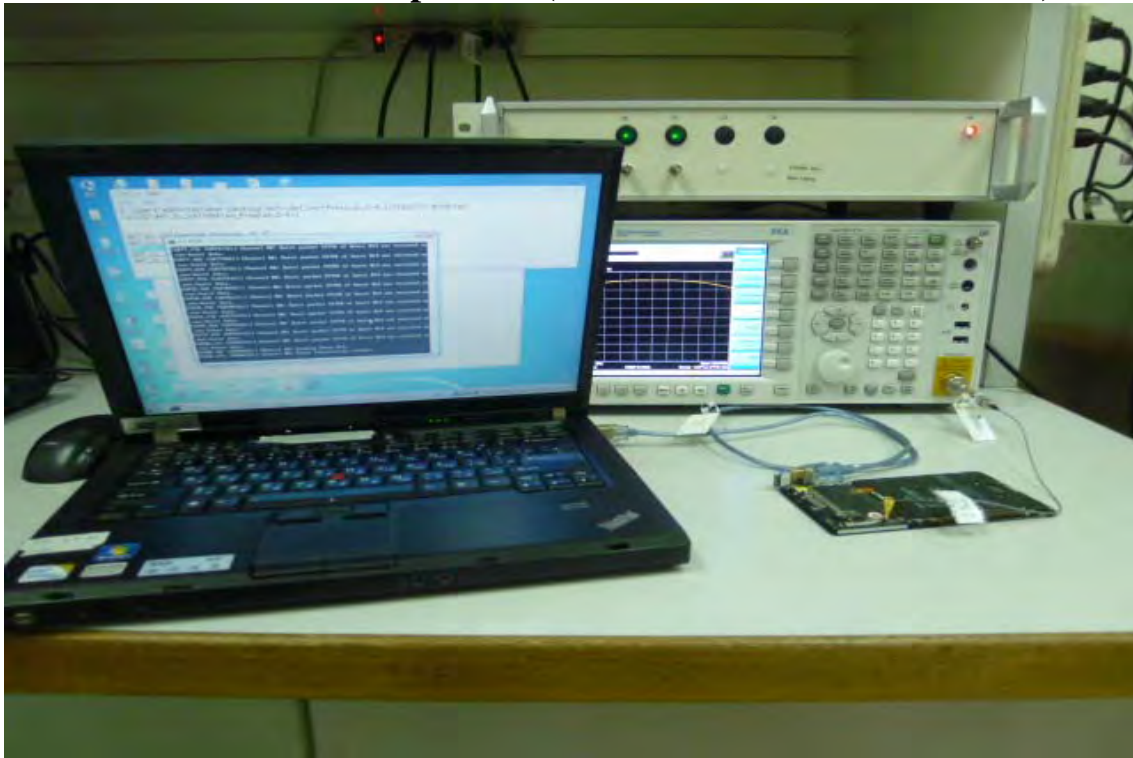
Conducted Setup Photo (Measurement at Antenna Port)
