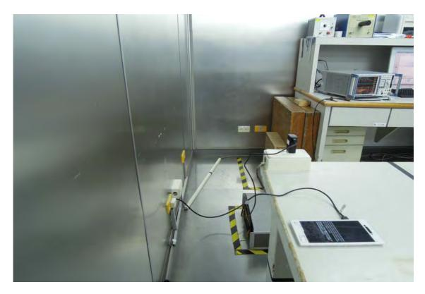
AC Power-line Conducted Emission Set up Photo (Adapter Model number: EP880)
