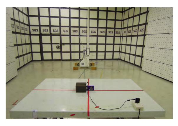
AC Power-line Conducted Emission Set up Photo (Adapter Model number: EP800)
