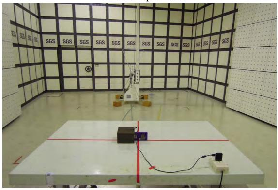
Radiated Emission Setup Photos (E1 Mode) Below 1GHz
