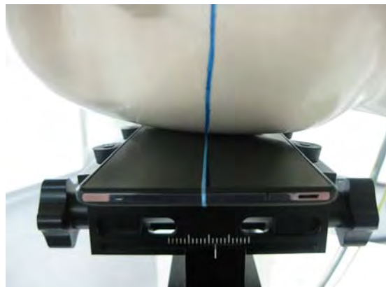
Fig.3 Right Head Section / Cheek-Touch Position
