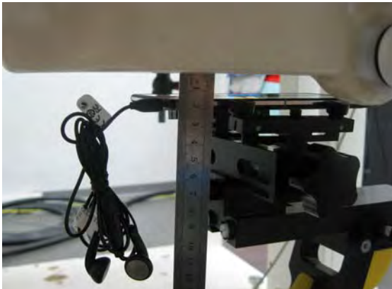
Fig.8 EUT front side with headset (MH410C) to flat phantom
