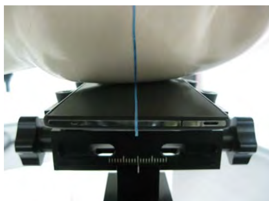
Fig.5 Left Head Section / Cheek-Touch Position
