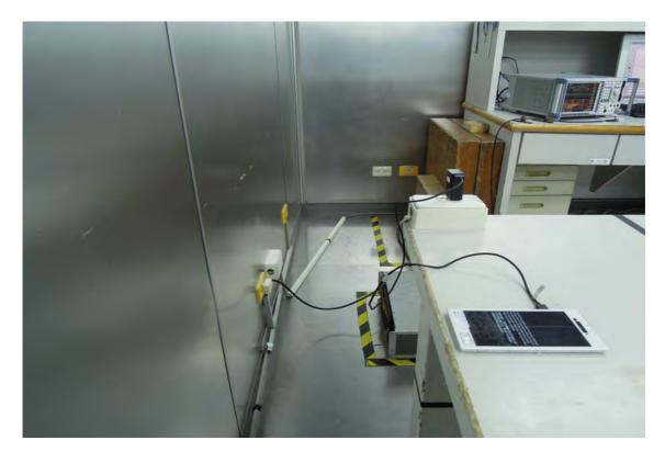
**Conducted Setup Photo (Measurement at Antenna Port)**
