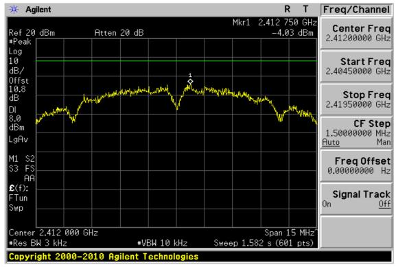
**Power Spectral Density Test Plot (CH-Mid)**
