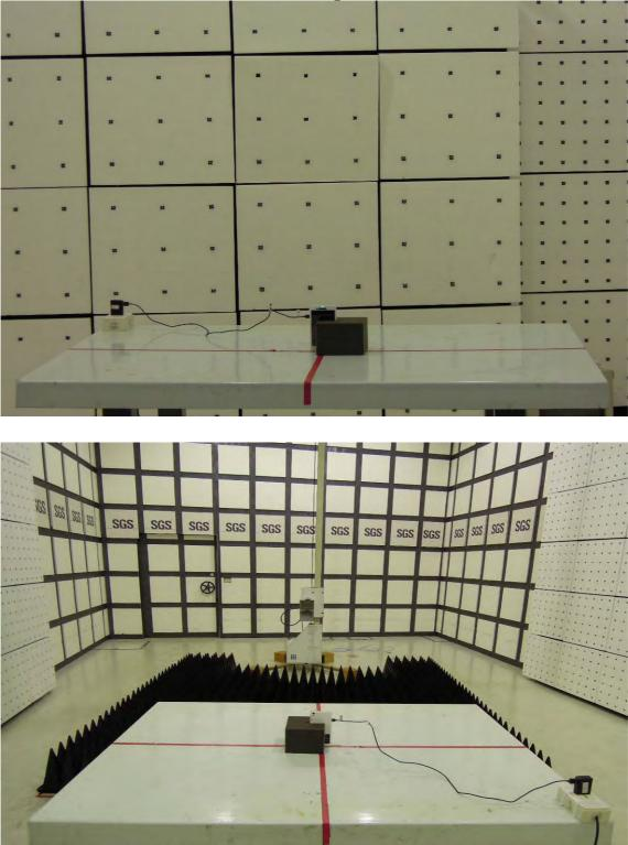
**Radiated Emission Set up Photos (H PLAN)**
