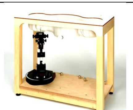
Fig 5.9 Photo of SAM Phantom
