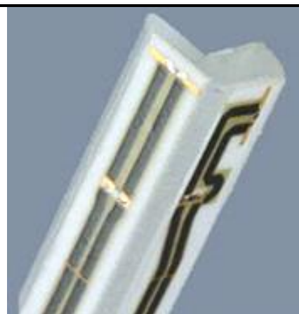
Fig 5.2 Photo of E-field Probe
