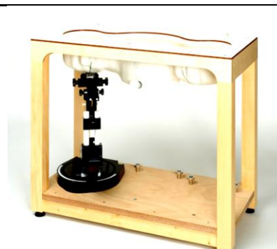
Fig 5.9 Photo of SAM Phantom
