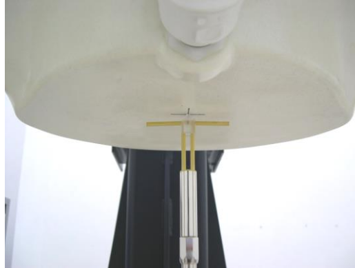
Fig 7.2 Photo of Dipole Setup
