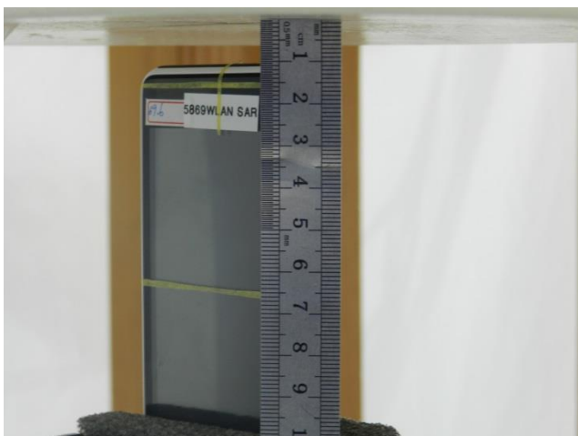
Top Side, Test Separation 1 cm
