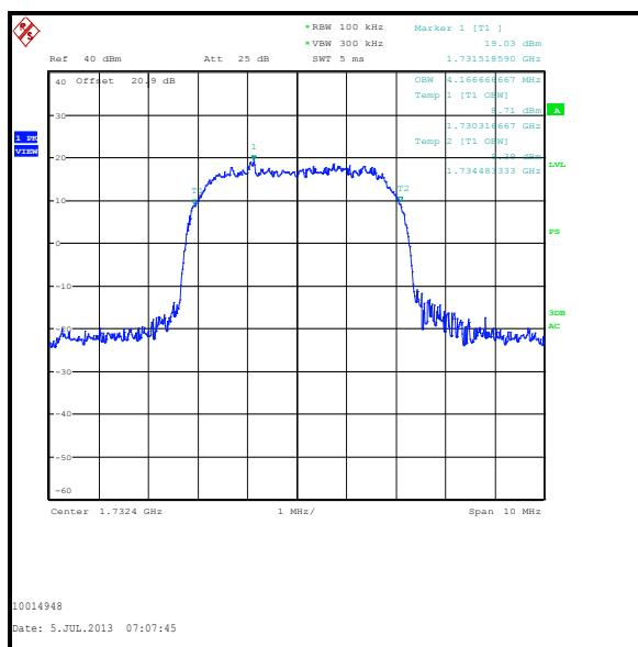
**Transmitter Occupied Bandwidth (continued)****Results: HSDPA Sub-Test 4**
