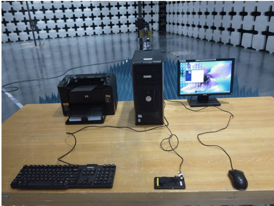
Pic.1 Radiated emission
