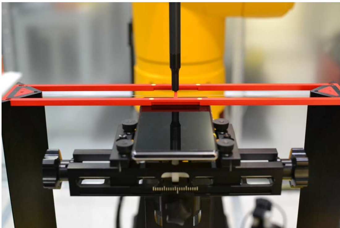
Figure 18-1 Ear Reference Point HAC Phantom Alignment
