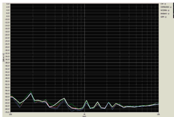
Figure 5-15 High power RF Emissions Effect with HAC Dipole on the T-coil Probe System 10mm between dipole maximum and magnetic probe
