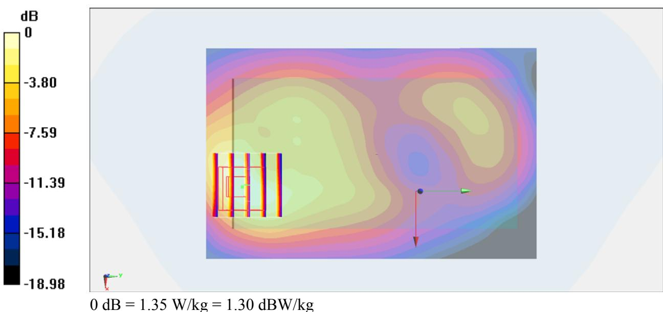
**#27\_GSM1900\_GPRS (4 Tx slots)\_Back\_1cm\_Ch810****DUT: 342505**
