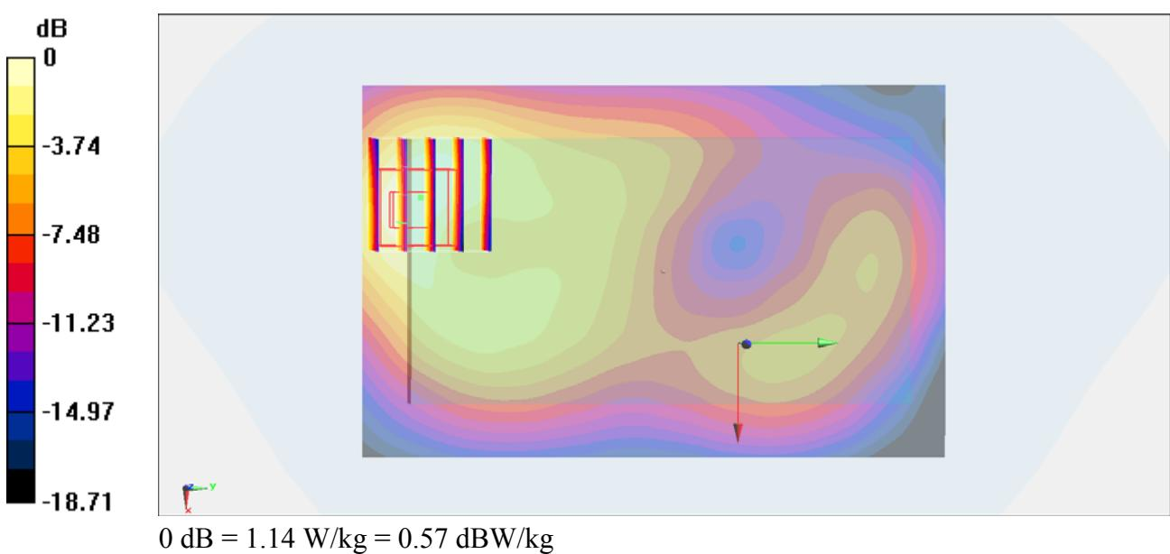
**#23\_GSM1900\_GPRS (4 Tx slots)\_Back\_1cm\_Ch512****DUT: 342505**
