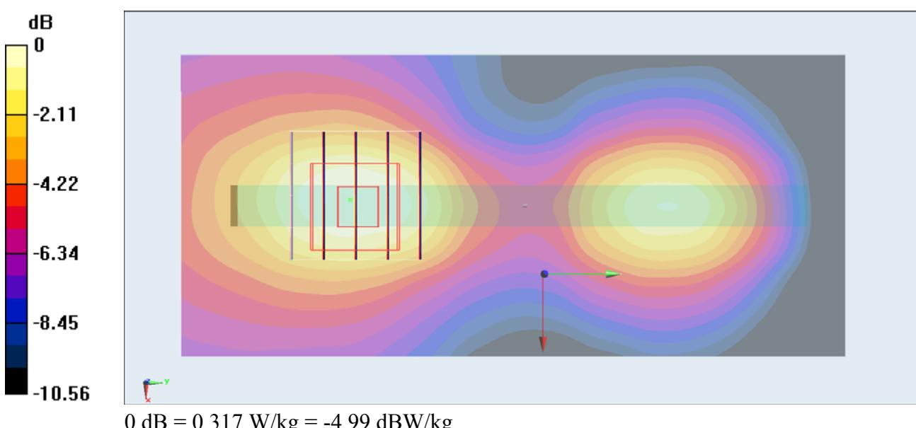
**#30\_GSM1900\_GPRS (4 Tx slots)\_Bottom Side\_1cm\_Ch512****DUT: 342505**
