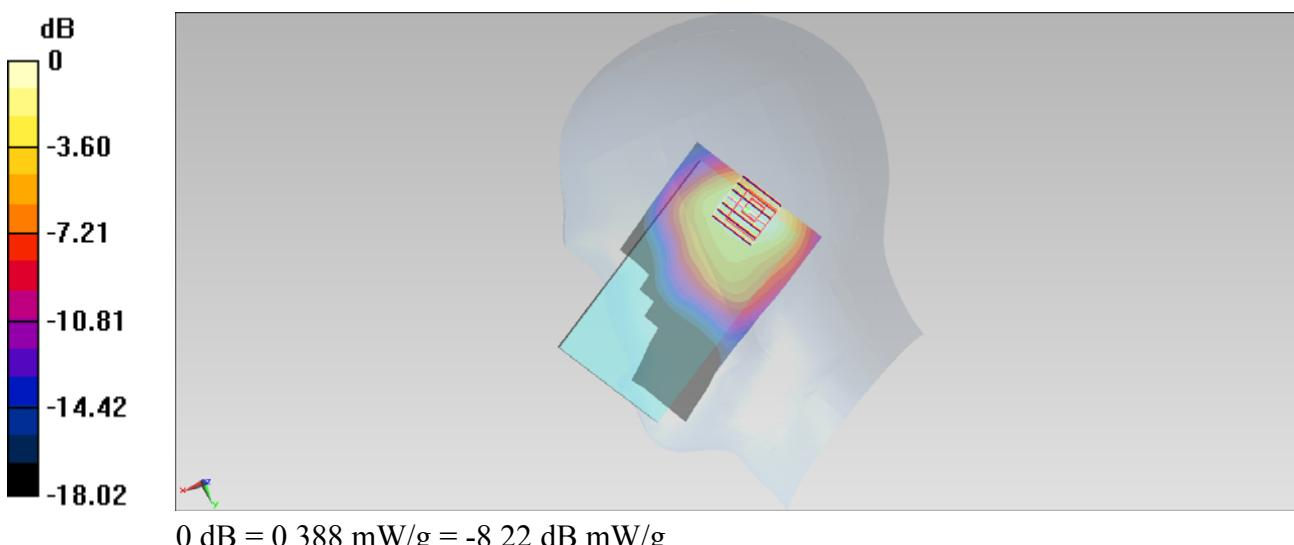
**#09\_WLAN2.4G\_802.11b 1Mbps\_Right Tilted\_Ch6****DUT: 342505**
