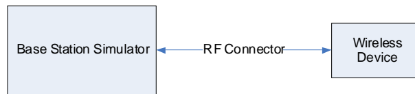
Figure 8-2 Power Measurement Setup
