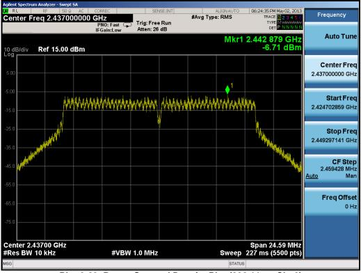
Plot 6-23. Power Spectral Density Plot (802.11g - Ch. 6)
