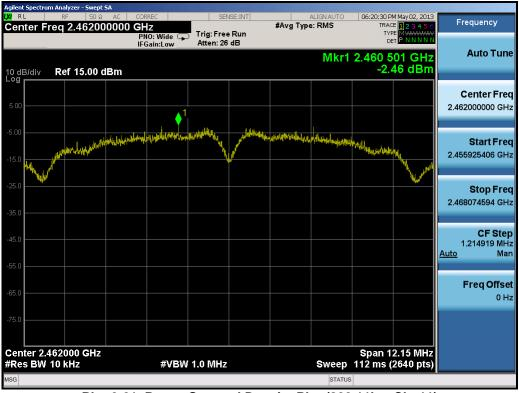
Plot 6-21. Power Spectral Density Plot (802.11b - Ch. 11)
