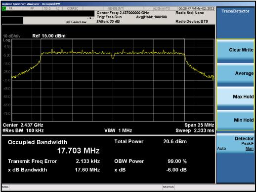
Plot 6-8. 6dB Bandwidth Plot (802.11n (2.4GHz) - Ch. 6)
