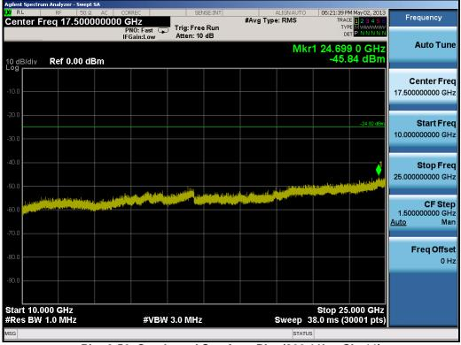
Plot 6-56. Conducted Spurious Plot (802.11b - Ch. 11)
