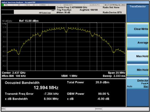
Plot 6-2. 6dB Bandwidth Plot (802.11b - Ch. 6)
