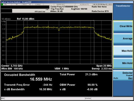
Plot 6-10. 6dB Bandwidth Plot (802.11a – Ch. 149)
