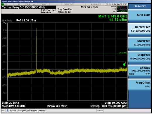
Plot 6-55. Conducted Spurious Plot (802.11b - Ch. 11)
