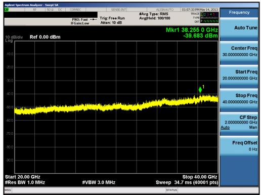
Plot 6-58. Conducted Spurious Plot (802.11a - Ch. 149)
