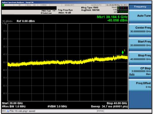
Plot 6-62. Conducted Spurious Plot (802.11a - Ch. 165)
