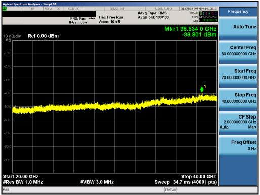
Plot 6-60. Conducted Spurious Plot (802.11a - Ch. 157)
