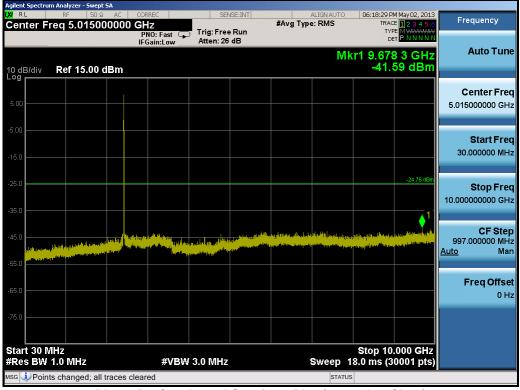
Plot 6-53. Conducted Spurious Plot (802.11b - Ch. 6)
