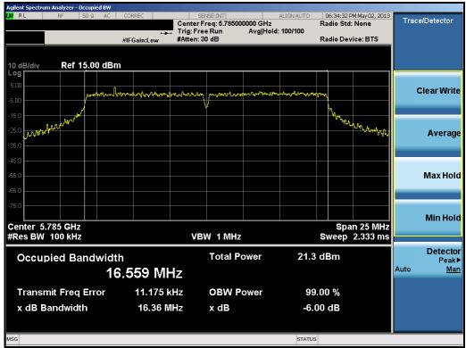
Plot 6-11. 6dB Bandwidth Plot (802.11a - Ch. 157)
