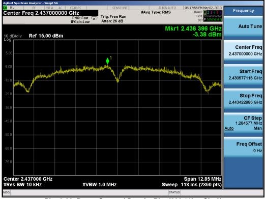
Plot 6-20. Power Spectral Density Plot (802.11b - Ch. 6)
