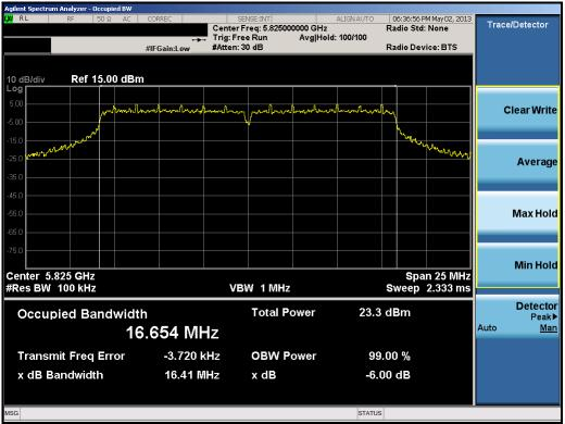
Plot 6-12. 6dB Bandwidth Plot (802.11a - Ch. 165)
