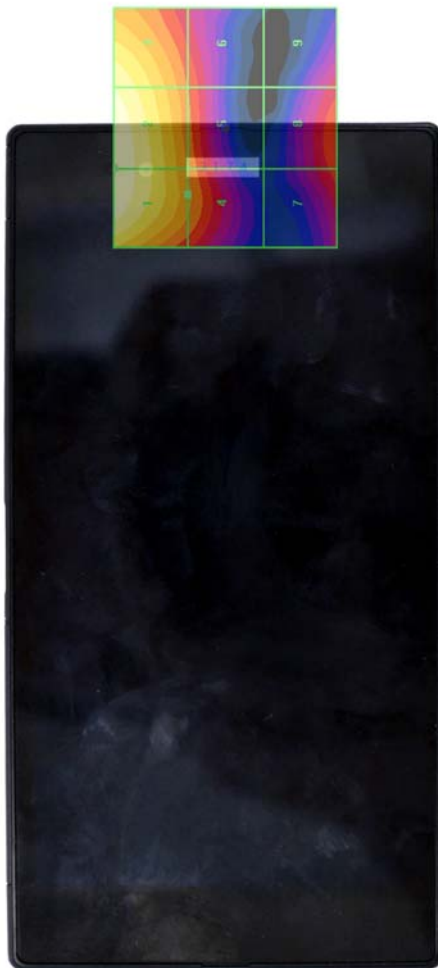
Figure 18-4 E-Field WD Scan overlay
