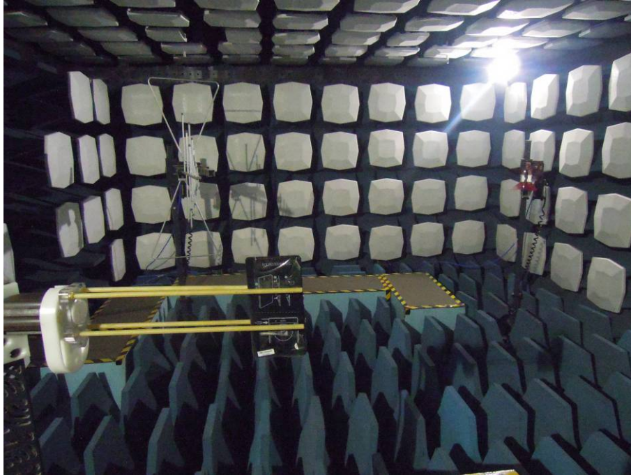
Pic.1 Radiated spurious emission
