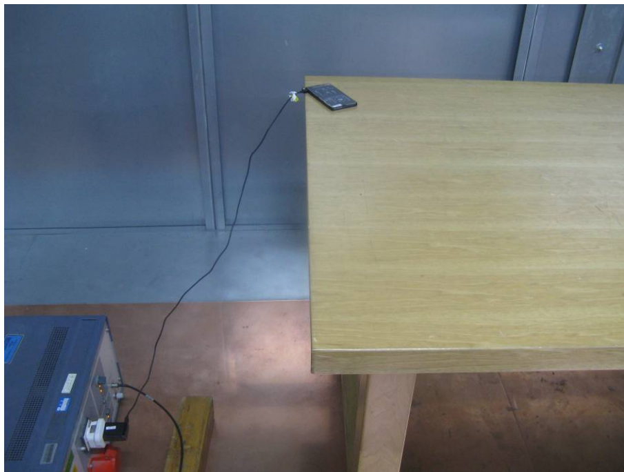
Pic.2 Conducted emission
