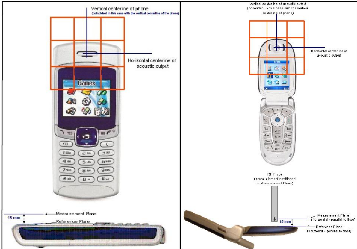
Figure 2 - WD reference and plane for RF emission measurements
