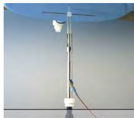
Photograph of the Dipole Antenna
