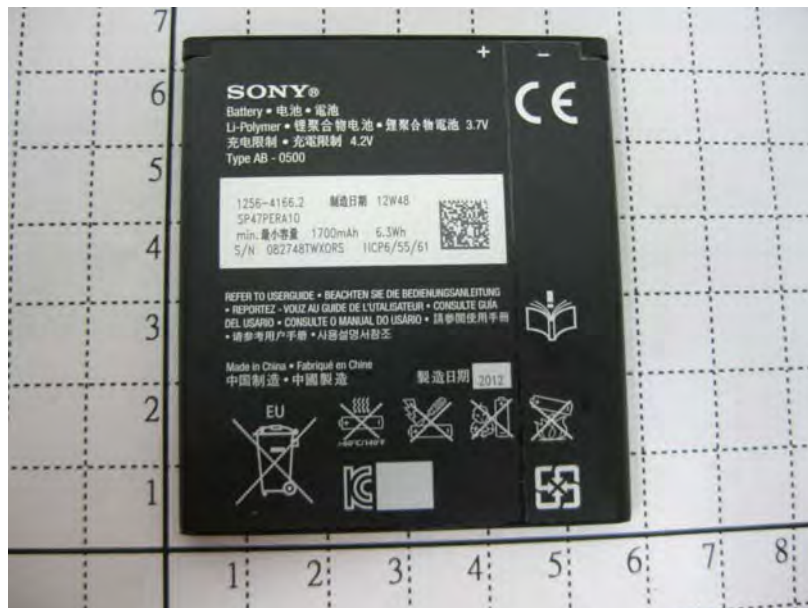
Fig.28 Back view of battery (Model No.: BA900, Supplier: SONY, Type No.: AB-0500)
