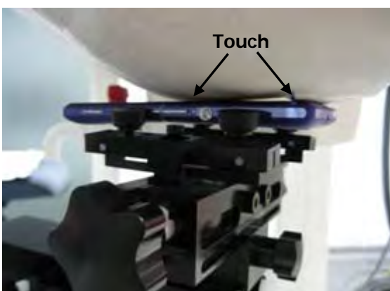
Fig.18 Left Head Section / Cheek-Touch Position
