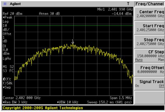
**Power Spectral Density Test Plot (CH-Mid)**
