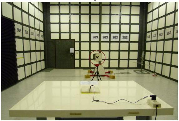
Antenna with V polarization
