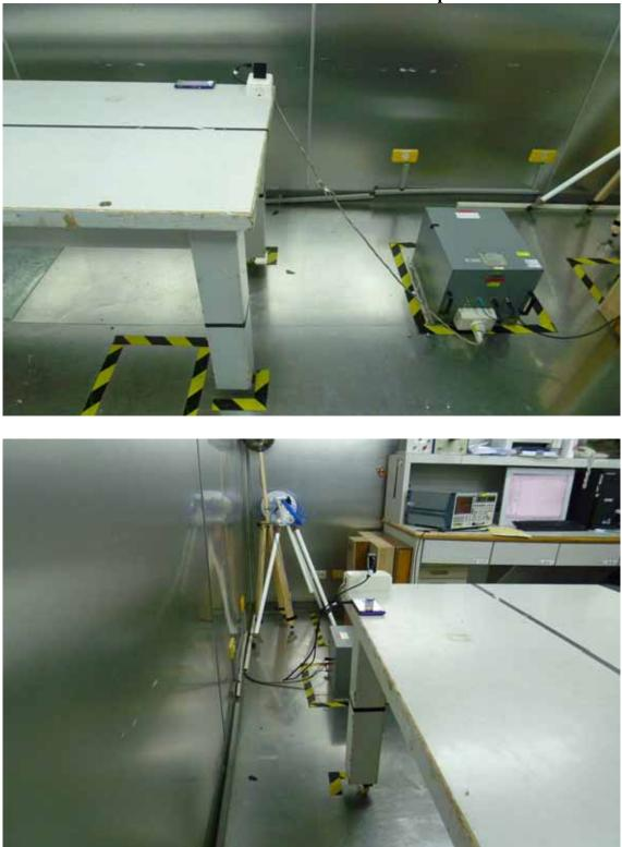
AC Power-line Conducted Emission Set up Photo
