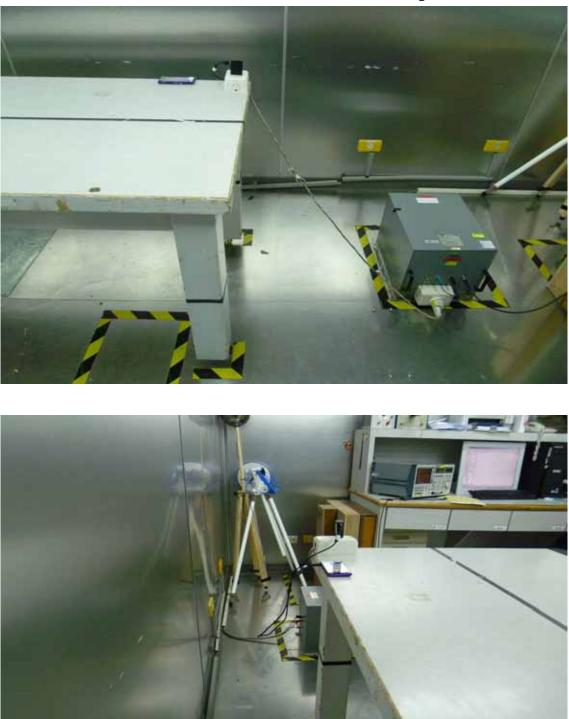
AC Power-line Conducted Emission Set up Photo
