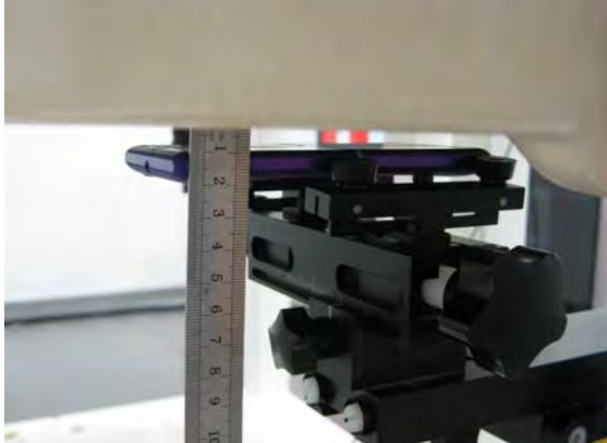
Fig.9 EUT front to flat phantom
