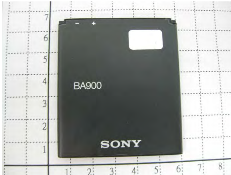
Fig.18 Front view of battery (Model No.: BA900, Supplier: SONY, Type No.: AB-0500)
