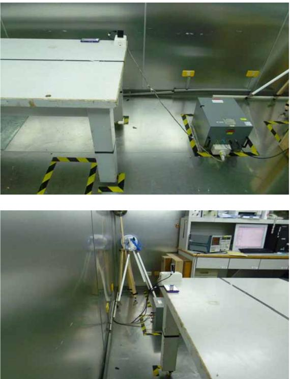
AC Power-line Conducted Emission Set up Photo
