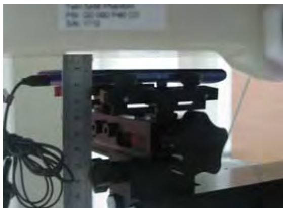
Fig.26 EUT front with headset (MH410C) to flat phantom
