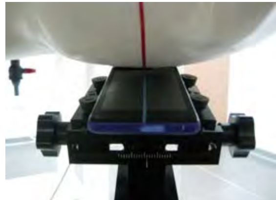
Fig.20 Left Head Section / Ear-Tilt Position(15°)
