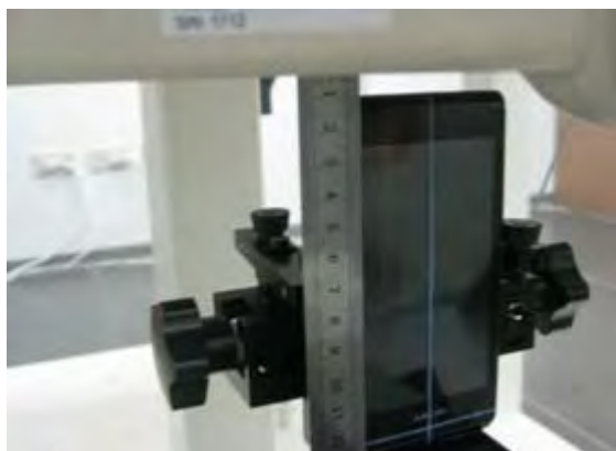
Fig.24 EUT bottom to flat phantom
