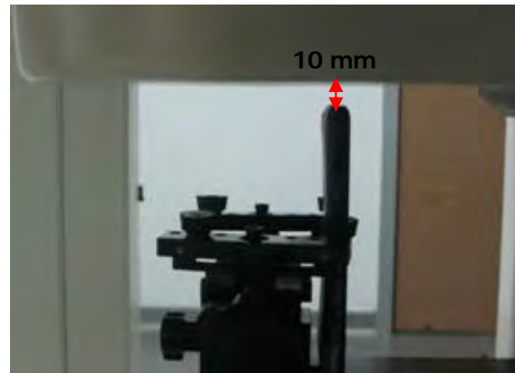
Fig.23 EUT top to flat phantom
