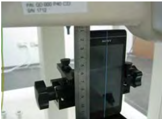
Fig.23 EUT top to flat phantom
