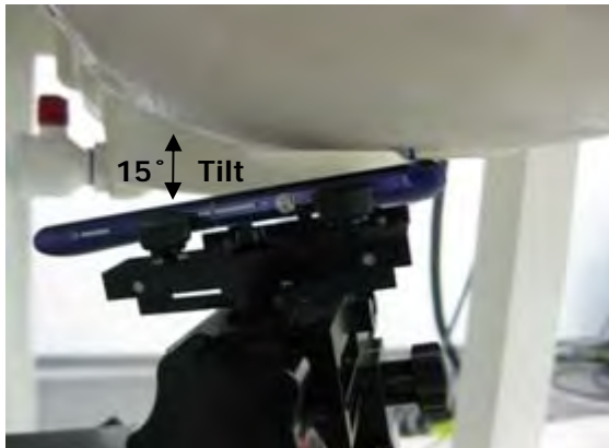
Fig.20 Left Head Section / Ear-Tilt Position(15°)
