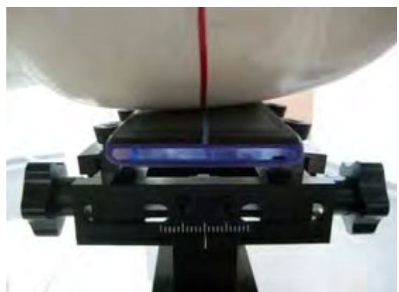
Fig.19 Left Head Section / Cheek-Touch Position
