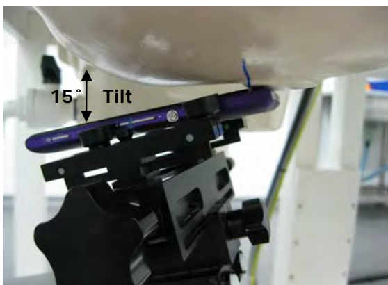
Fig.6 Left Head Section / Ear-Tilt Position(15°)
