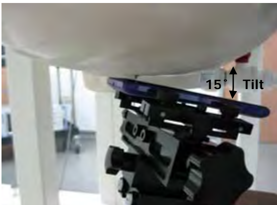
Fig.18 Right Head Section / Ear-Tilt Position(15°)
