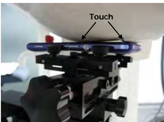
Fig.19 Left Head Section / Cheek-Touch Position
