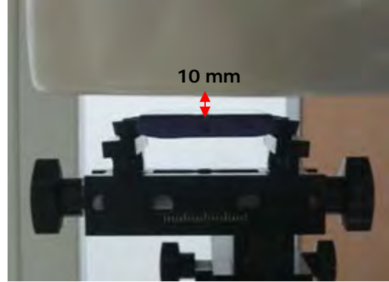
Fig.21 EUT front to flat phantom
