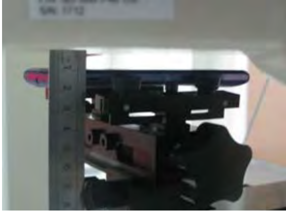
Fig.21 EUT front to flat phantom
