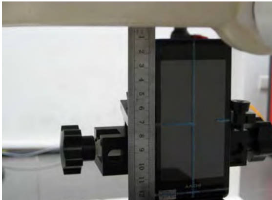
Fig.14 EUT bottom to flat phantom
