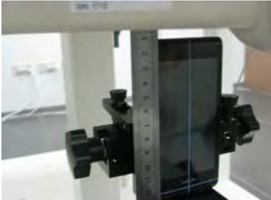
Fig.24 EUT bottom to flat phantom
