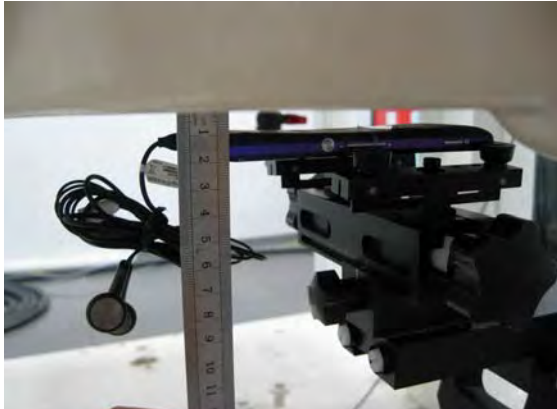
Fig.12 EUT back with headset (MH410C) to flat phantom
