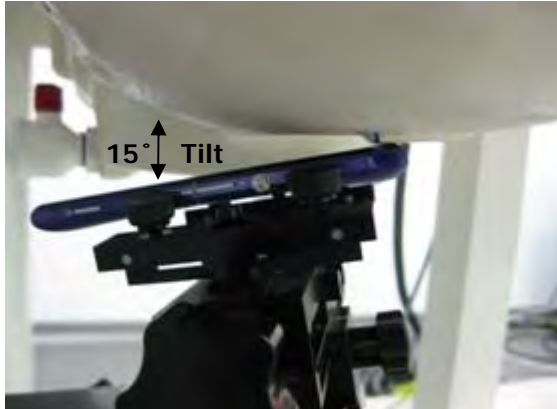
Fig.20 Left Head Section / Ear-Tilt Position(15°)
