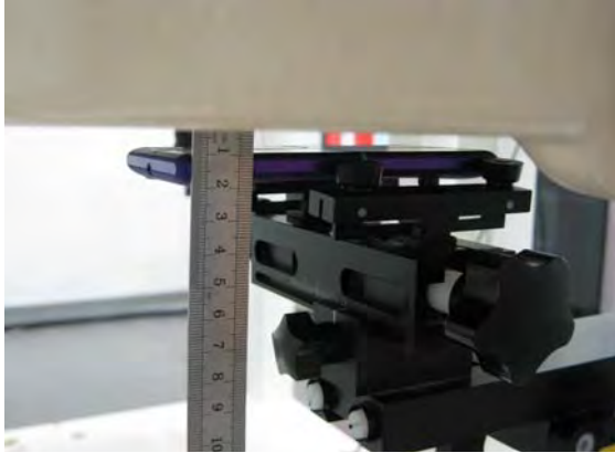
Fig.9 EUT front to flat phantom
