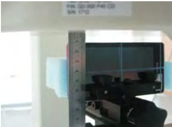
Fig.25 EUT left to flat phantom
