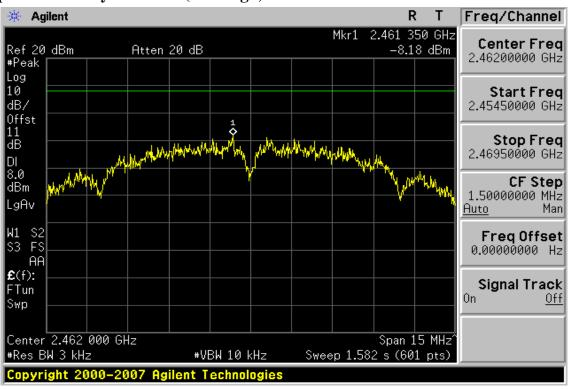
802.11g **Power Spectral Density Test Plot (CH-Low)**
