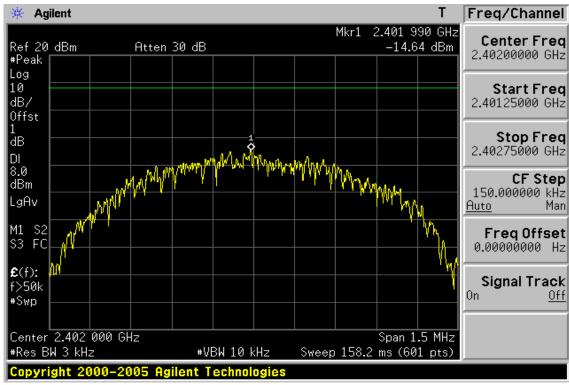
**Power Spectral Density Test Plot (CH-Mid)**
