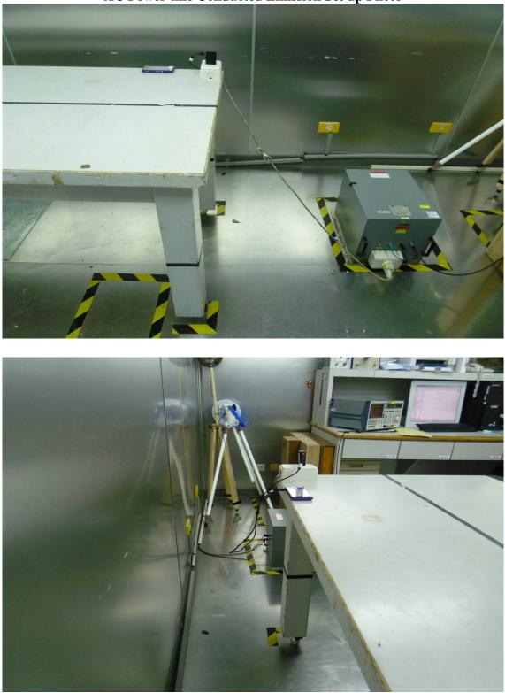
AC Power-line Conducted Emission Set up Photo
