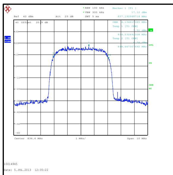
**Transmitter Occupied Bandwidth (continued)****Results: HSUPA Sub-Test 3**
