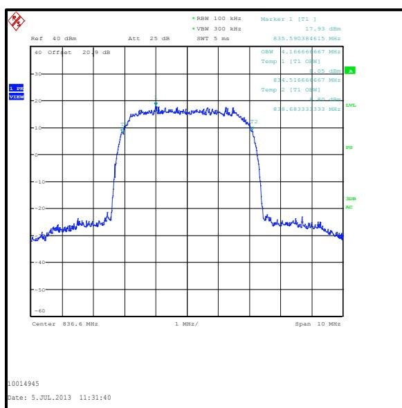
**Transmitter Occupied Bandwidth (continued)****Results: HSDPA Sub-Test 1**
