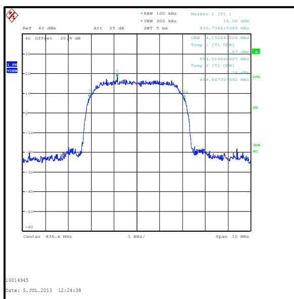
**Transmitter Occupied Bandwidth (continued)****Results: HSDPA Sub-Test 4**
