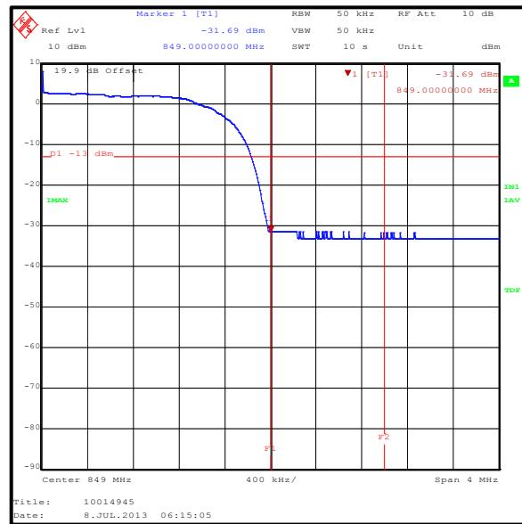
**Transmitter Radiated Emissions at Band Edges (continued)****Results: HSDPA Sub-Test 1**
