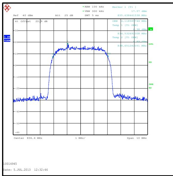
**Transmitter Occupied Bandwidth (continued)****Results: HSUPA Sub-Test 2**
