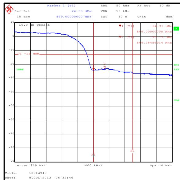
**Transmitter Radiated Emissions at Band Edges (continued)****Results: HSDPA Sub-Test 3**
