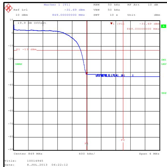
**Transmitter Radiated Emissions at Band Edges (continued)****Results: HSUPA Sub-Test 5**
