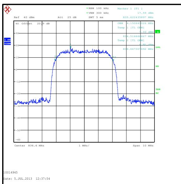
**Transmitter Occupied Bandwidth (continued)****Results: HSUPA Sub-Test 4**
