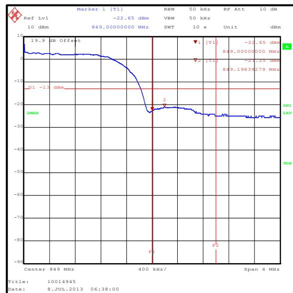
**Transmitter Radiated Emissions at Band Edges (continued)****Results: HSUPA Sub-Test 1**
