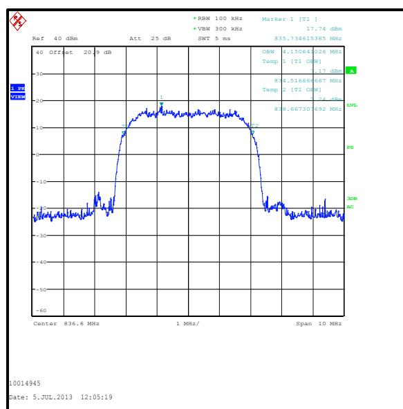
**Transmitter Occupied Bandwidth (continued)****Results: HSUPA Sub-Test 1**
