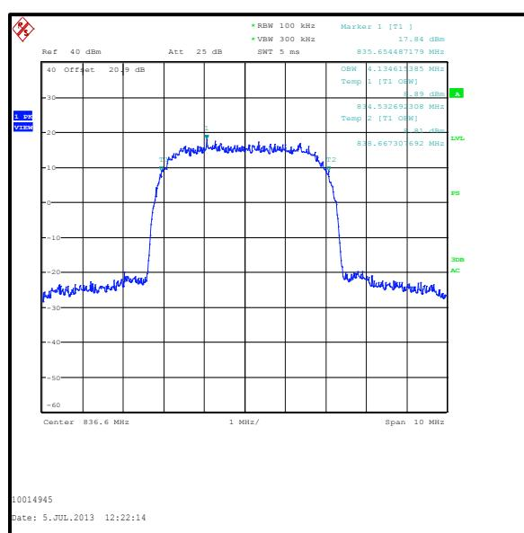
**Transmitter Occupied Bandwidth (continued)****Results: HSDPA Sub-Test 3**
