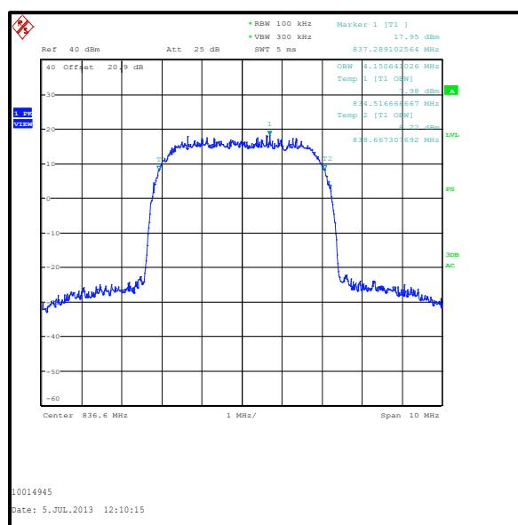
**Transmitter Occupied Bandwidth (continued)****Results: HSDPA Sub-Test 2**
