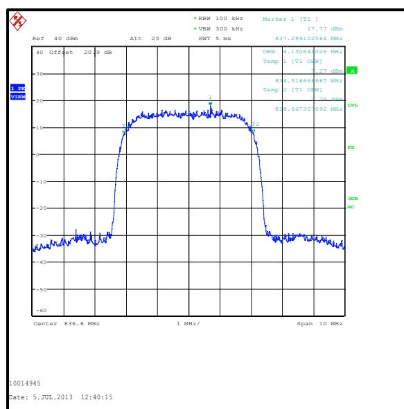
**Transmitter Occupied Bandwidth (continued)****Results: HSUPA Sub-Test 5**
