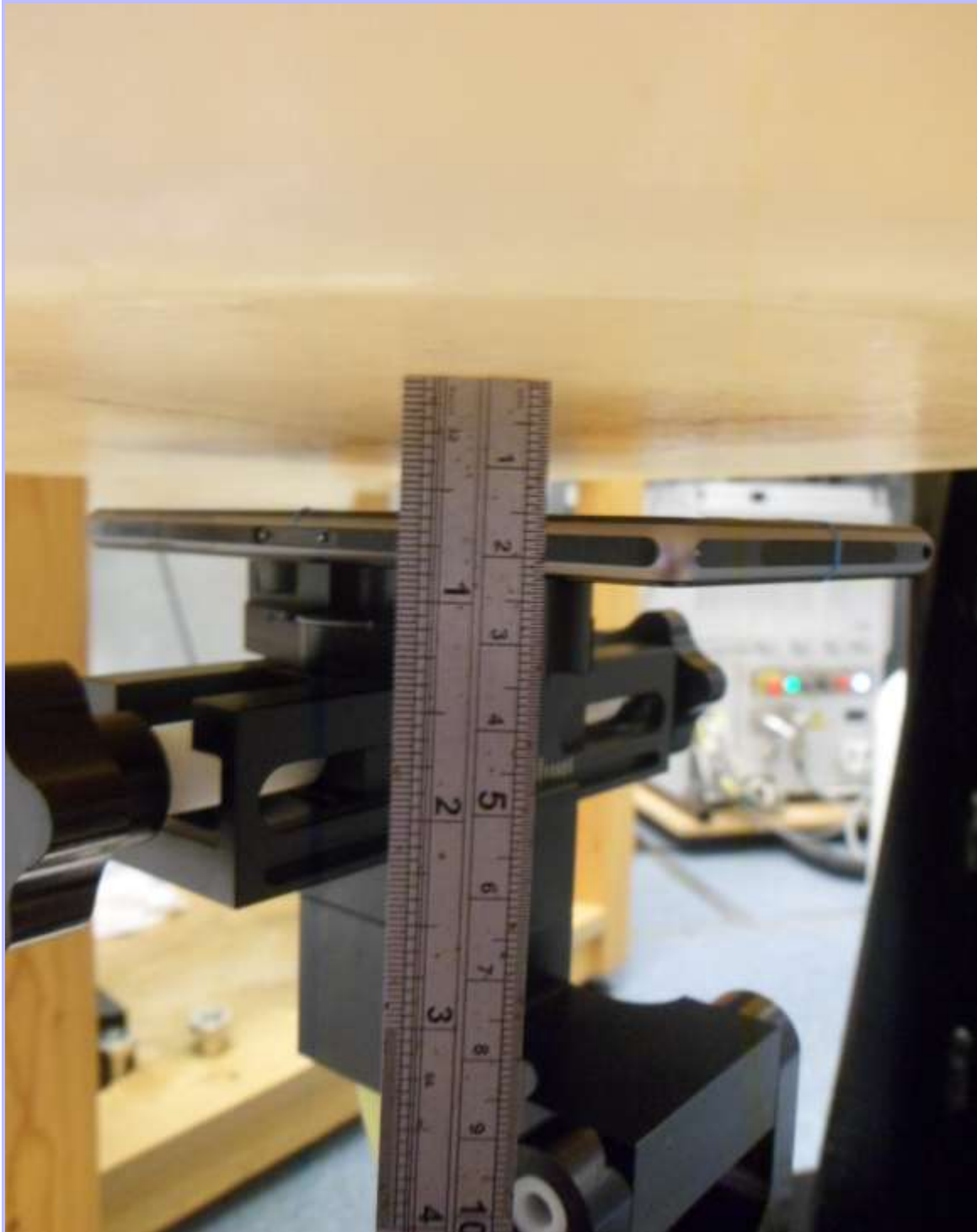
PHT/10014935/007: Front of EUT Facing Phantom at 15mm
