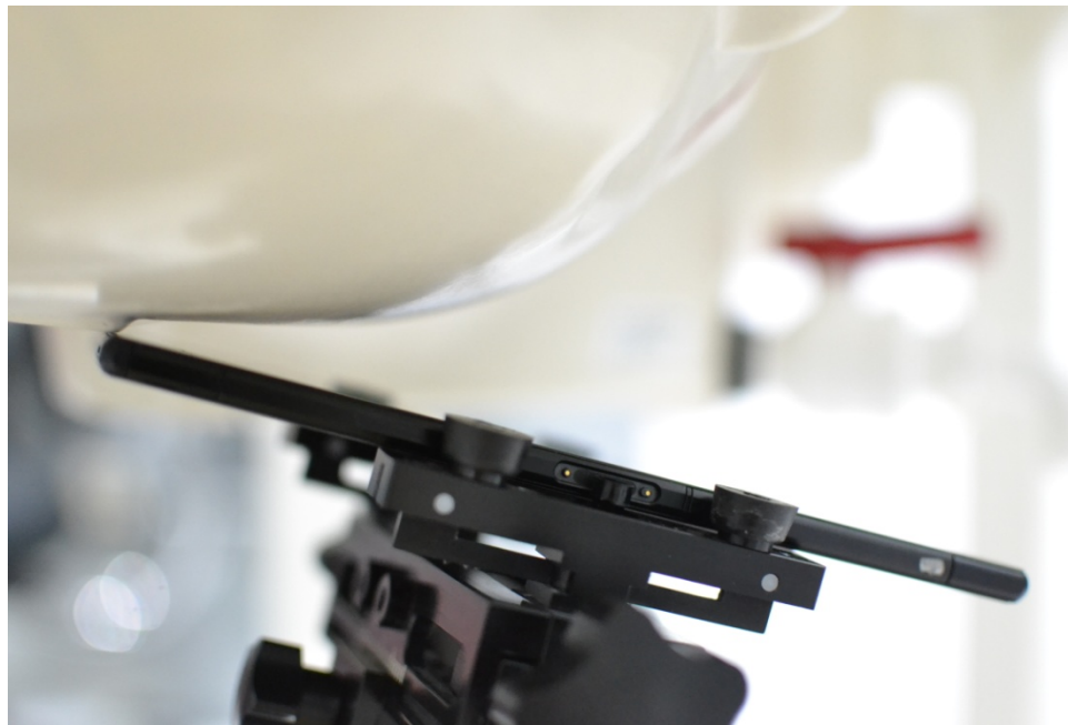
SAR Test Setup Photo 2 – Right Tilt
