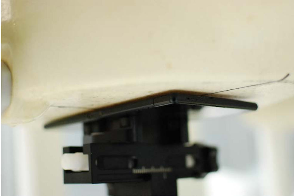
SAR Test Setup Photo 13 – Back Side at 0.3 cm
