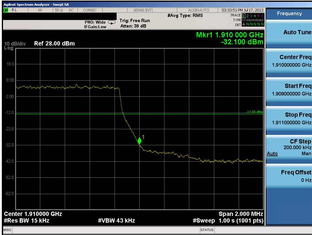
Plot 10-5. Upper Band Edge Plot (1.4MHz QPSK – RB Size 6)
