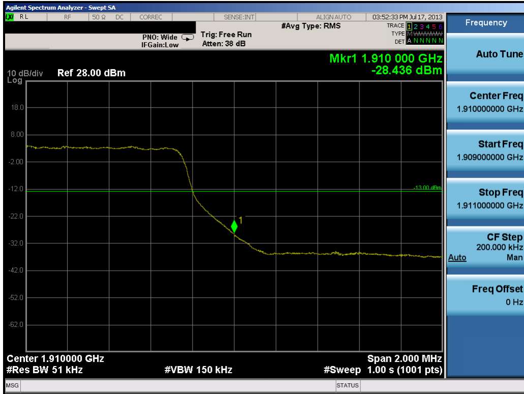
Plot 10-21. Upper Band Edge Plot (5.0MHz QPSK – RB Size 25)
