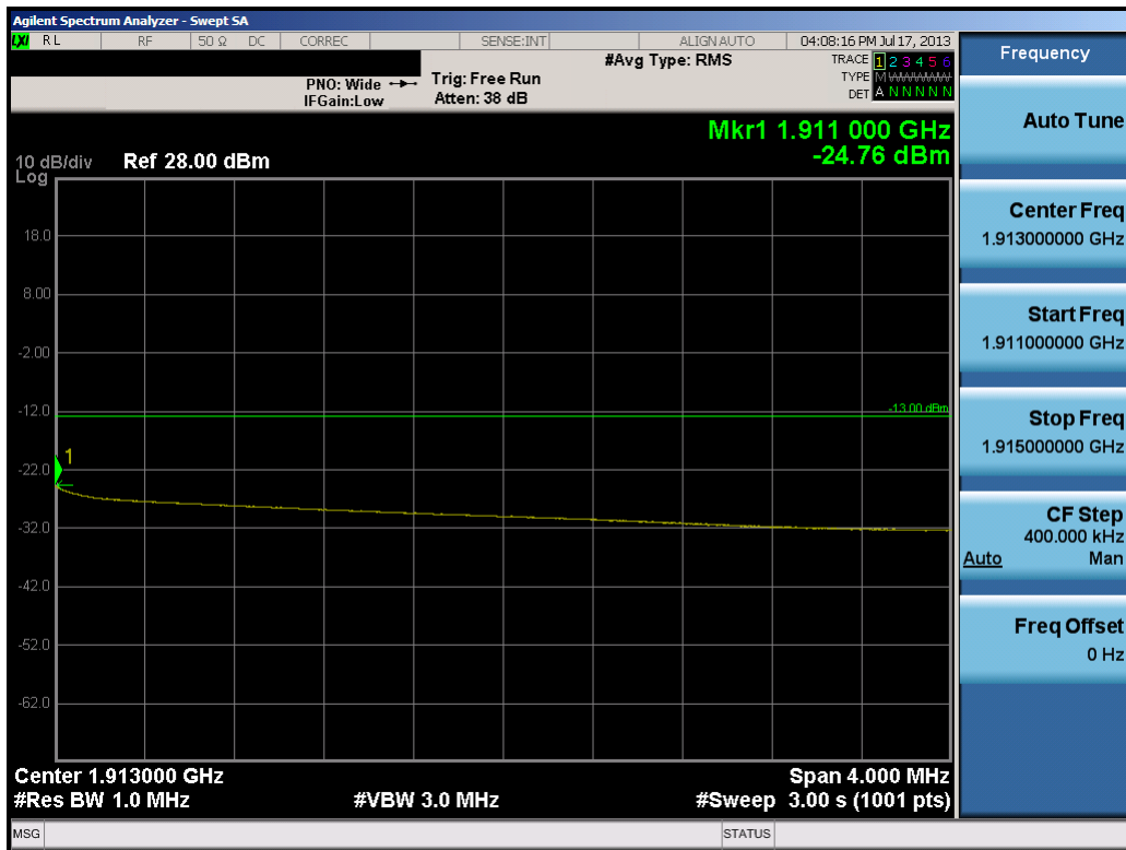
Plot 10-30. Upper Extended Band Edge Plot (10.0MHz QPSK – RB Size 50)
