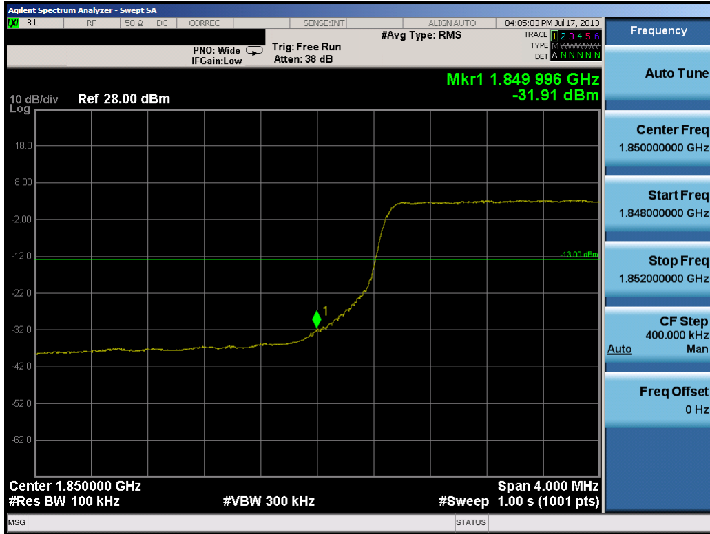
Plot 10-25. Lower Band Edge Plot (10.0MHz QPSK – RB Size 50)
