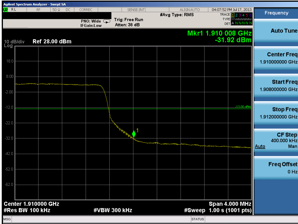
Plot 10-29. Upper Band Edge Plot (10.0MHz QPSK – RB Size 50)
