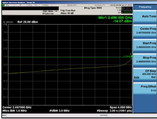
Plot 10-3. Lower Extended Band Edge Plot (5.0MHz QPSK - RB Size 25)
