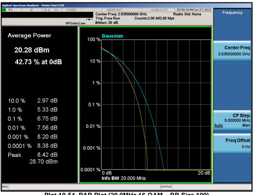
Plot 10-54. PAR Plot (20.0MHz 16-QAM - RB Size 100)
