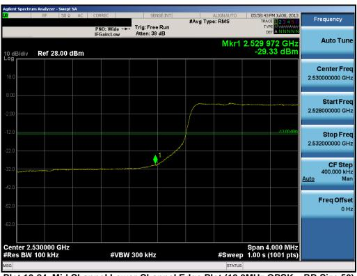
Plot 10-24. Mid Channel Lower Channel Edge Plot (10.0MHz QPSK - RB Size 50)
