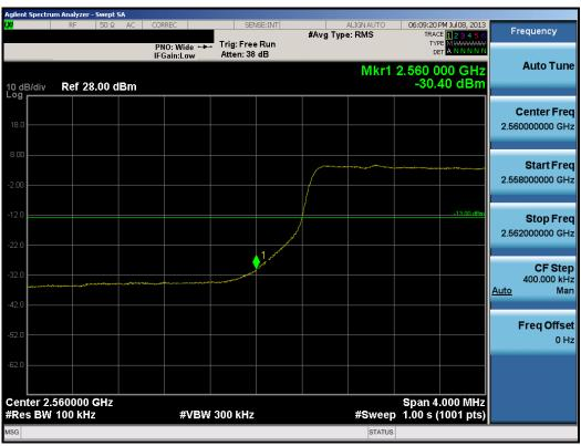
Plot 10-26. Low Channel Lower Channel Edge Plot (10.0MHz QPSK - RB Size 50)
