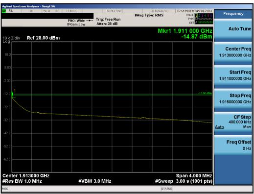
Plot 9-28. Upper Extended Band Edge Plot (5.0MHz QPSK - RB Size 25)
