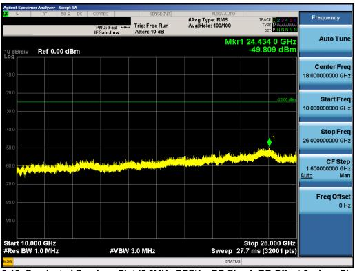
Plot 10-12. Conducted Spurious Plot (5.0MHz QPSK - RB Size 1, RB Offset 0 - Low Channel)
