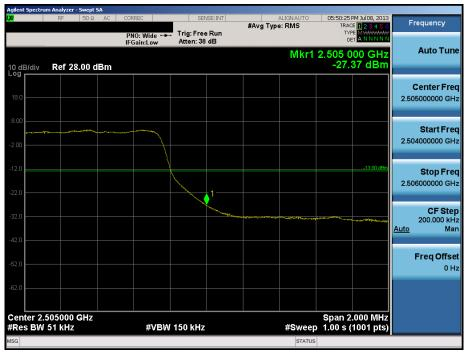
Plot 10-2. Low Channel Upper Channel Edge Plot (5.0MHz QPSK – RB Size 25)
