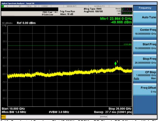
Plot 10-16. Conducted Spurious Plot (5.0MHz QPSK - RB Size 1, RB Offset 0 - High Channel)
