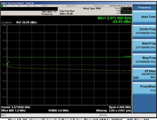
Plot 10-28. Upper Extended Band Edge Plot (10.0MHz QPSK - RB Size 50)
