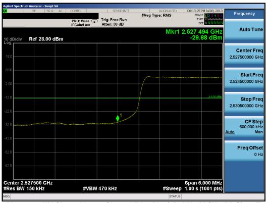
Plot 10-36. Mid Channel Lower Channel Edge Plot (15.0MHz QPSK - RB Size 75)
