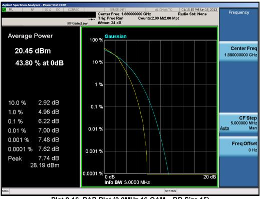
Plot 9-16. PAR Plot (3.0MHz 16-QAM - RB Size 15)
