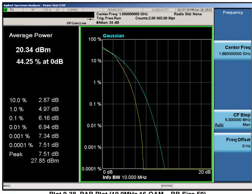
Plot 9-38. PAR Plot (10.0MHz 16-QAM - RB Size 50)
