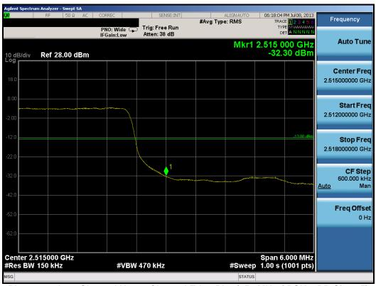
Plot 10-32. Low Channel Upper Channel Edge Plot (15.0MHz QPSK - RB Size 75)
