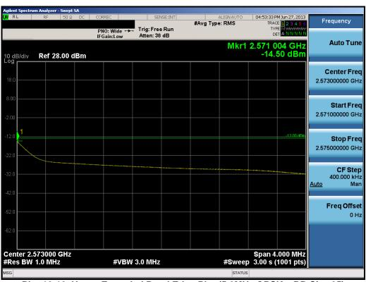
Plot 10-10. Upper Extended Band Edge Plot (5.0MHz QPSK - RB Size 25)
