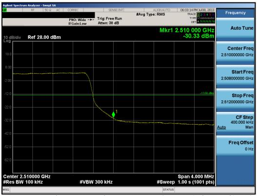
Plot 10-20. Low Channel Upper Channel Edge Plot (10.0MHz QPSK - RB Size 50)
