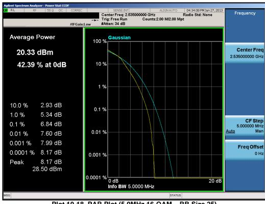
Plot 10-18. PAR Plot (5.0MHz 16-QAM - RB Size 25)
