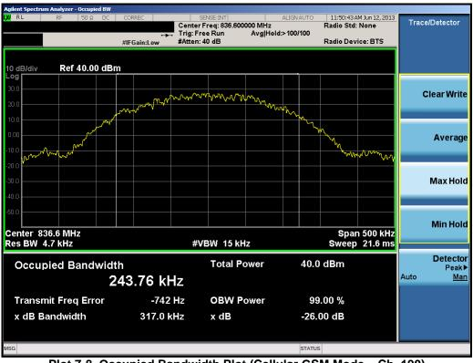
Plot 7-8. Occupied Bandwidth Plot (Cellular GSM Mode - Ch. 190)
