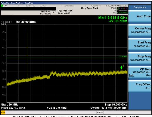
Plot 7-38. Conducted Spurious Plot (AWS WCDMA Mode - Ch. 1312)
