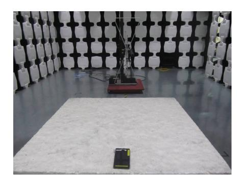
**Layout of AC Powerline Conducted Emission**
