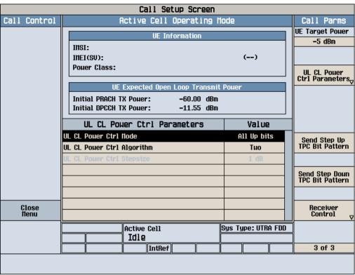
Figure 4: UL CL Power Ctrl Parameters
