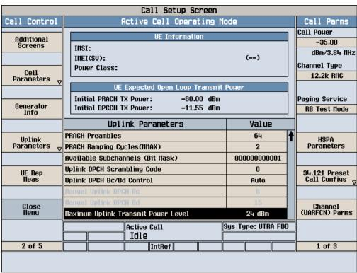
Figure 6: Uplink Parameters
