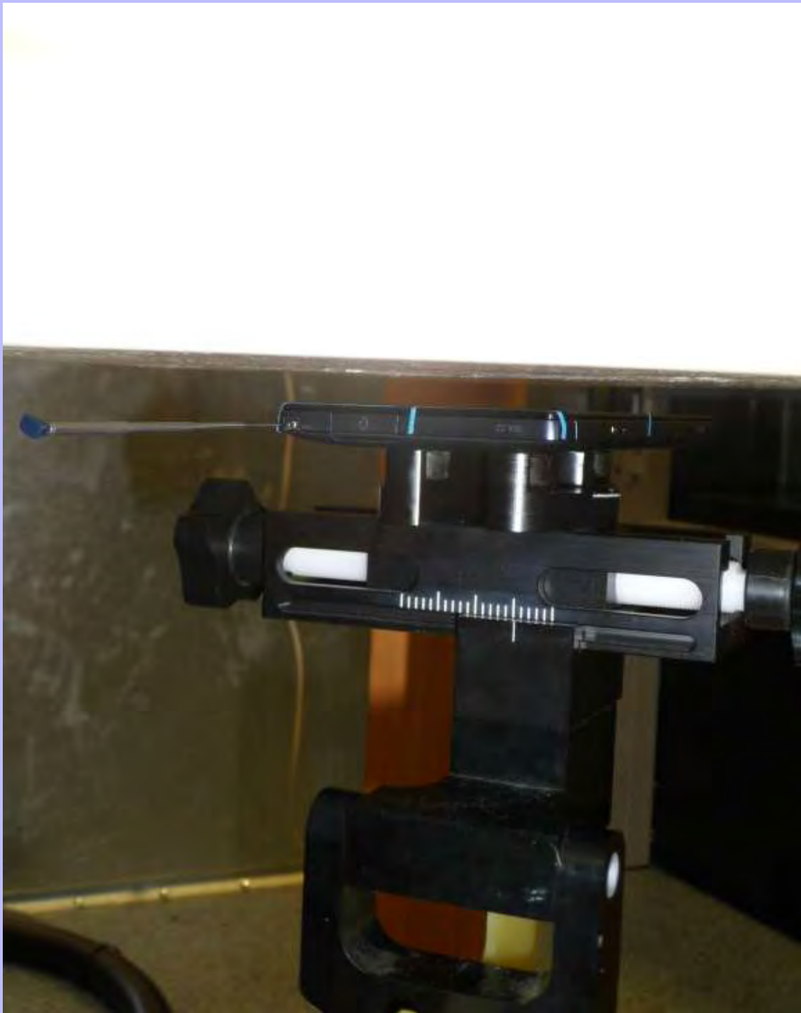
PHT/92490/010: Front of EUT Facing Phantom Antenna Extended at 10mm
