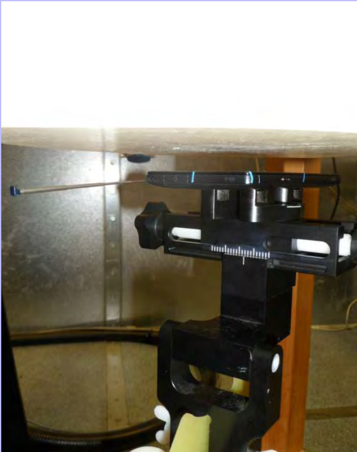
PHT/92490/012: Front of EUT Facing Phantom Antenna Extended at 15mm
