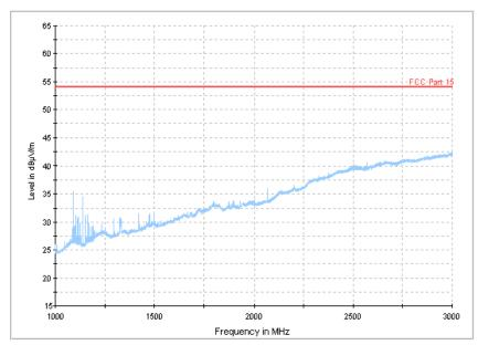
Figure B.2 Radiated Emission from 1GHz to 3GHz
