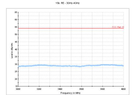
Figure B.3 Radiated Emission from 3GHz to 4GHz
