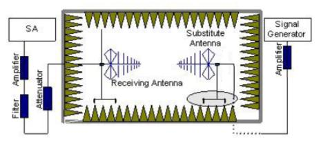
In the chamber, a substitution antenna for the frequency band of interest is placed at the reference point of the chamber. An RF signal source for the frequency band of interest is
